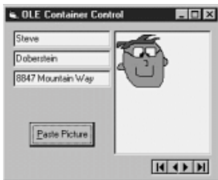
Figure 10.10: Graphical information acquired from an image-editing program and pasted into the database using the OLE Container control.
