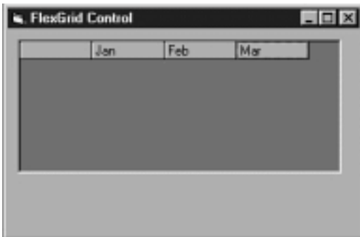
Figure 12.2 Using the Row Col and Text properties to populate the grid header.
