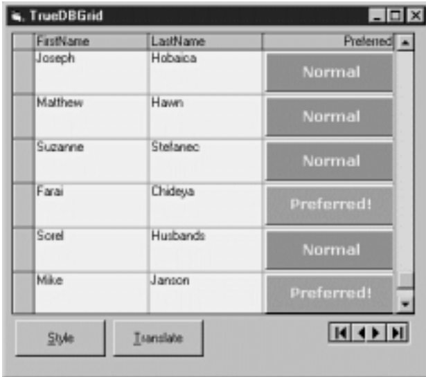
Figure 11.18: Grid displaying a graphic instead of a text value in a column.
