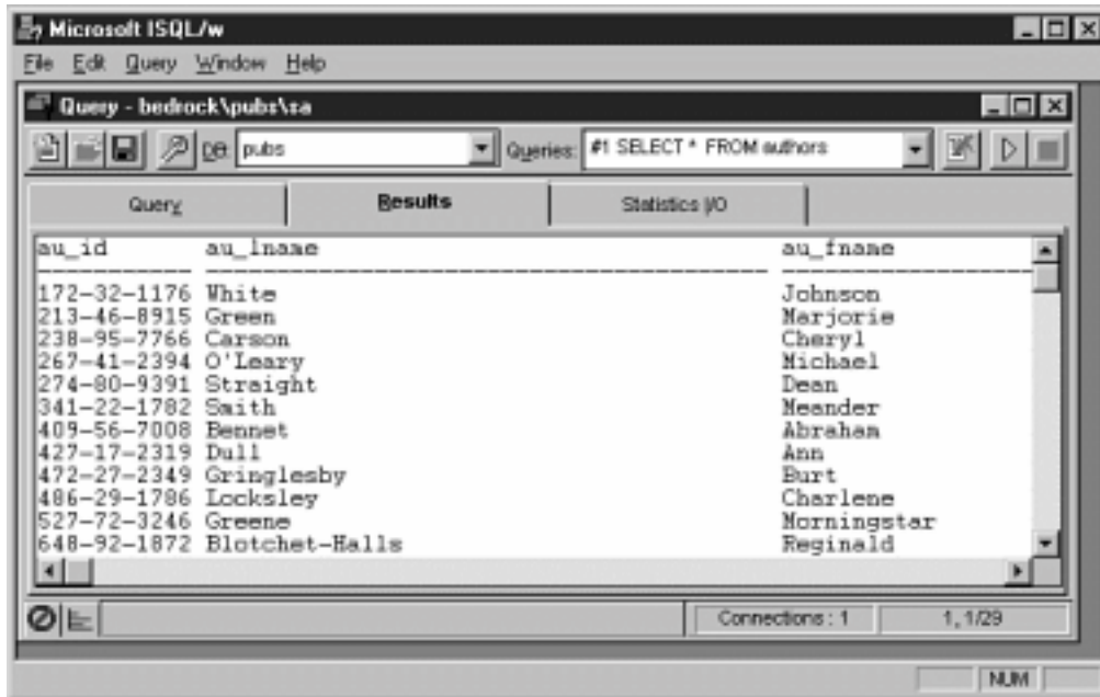
Figure 5.13: Results of a test query against the pubs database as displayed in the ISQL/w window.
