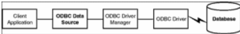
Figure 5.30: ODBC architecture showing the connection between the client application and the server database through the ODBC Driver Manager.
