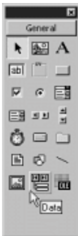
Figure 1.33: The Visual Basic Data control as it appears in the Visual Basic toolbox.
