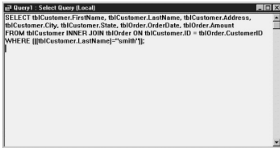
Figure 2.19: Microsoft Access gives the ability to view the SQL behind a Query Design.
