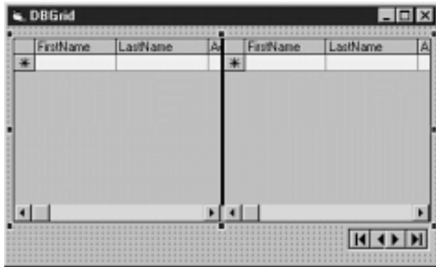
Figure 11.9: A vertical split created at design time.
