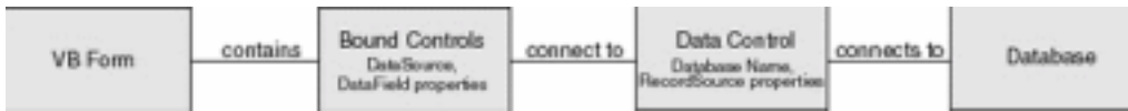
Figure 1.32: The components involved in connecting a Visual Basic application to a database through the Data control.
