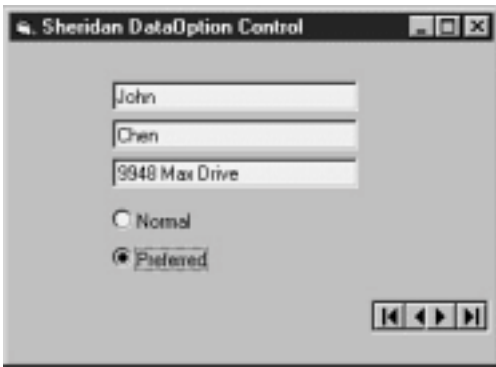
Figure 13.15: The DataOption control at runtime displaying the contents of the TypeID field.
